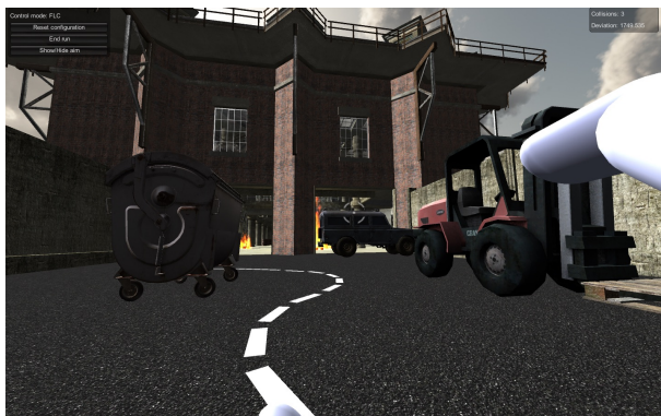
Fig. 4. Screen shot from the Path following scenario. The operator should reach the end of the dashed path as fast as possible, without colliding with moving or static obstacles, or deviating too much from the path.
